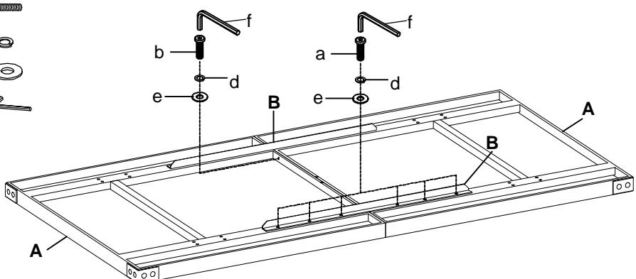
Step 2. Loosely attach the leg frames (C) to the assembled table tops (A) as shown below. Securely tighten all bolts with Allen wrench (f).
