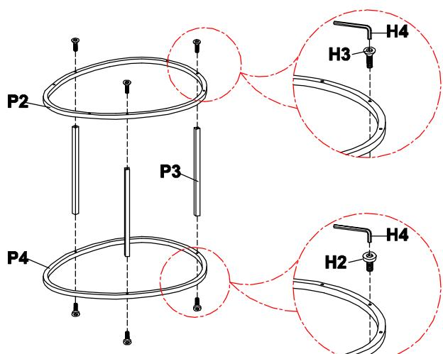
**Step 2.** Attach the assembled base to the bottom of table top (P1) as shown below. Securely tighten all bolts with Allen wrench (H4).
