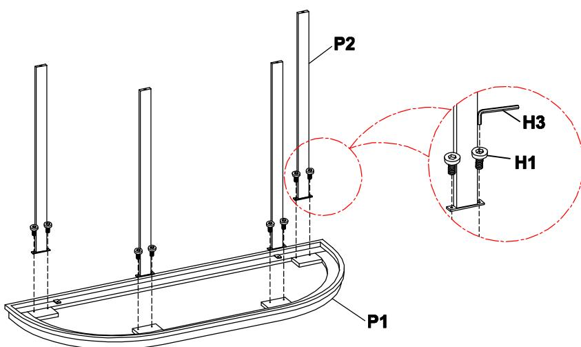
**Step 2.** Attach bottom frame (P3) to the bottom of posts (P2) as shown below. Securely tighten all bolts with Allen wrench (H3).
