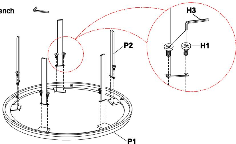
**Step 2.** Attach bottom frame (P3) to the bottom of post (P2) as shown below. Securely tighten all bolts with Allen wrench (H3).
