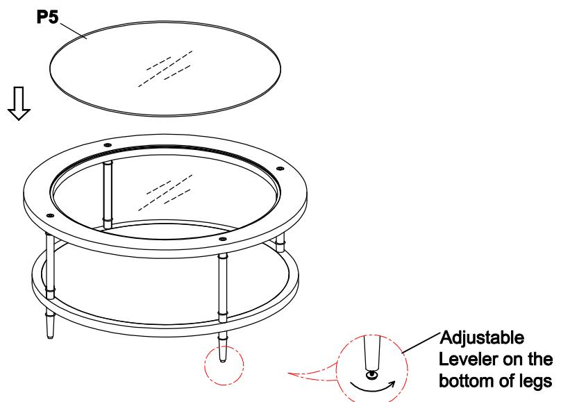
ADDITIONAL NOTE ABOUT SAFETY: BOLTS MAY LOOSEN DURING NORMAL EVERYDAY USE. THEY SHOULD BE PERIODICALLY INSPECTED AND RE-TIGHTENED TO PREVENT DAMAGE OR INJURY. ALWAYS CHECK TO BE SURE THAT ALL HARDWARE IS KEPT TIGHTENED.
