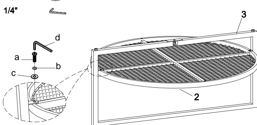
Step 2. Attach the leg2 (4) to assembled leg1(3) as shown below.
