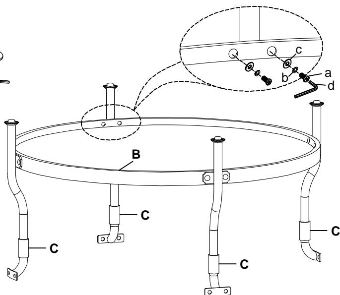
Step 2. Attach each assembled leg (C) to the table top frame (A) as shown below. Securely tighten all bolts with Allen wrench (d).
