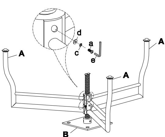
Step 2. Attach the assembled Legs (A) and center post (B) to the top panel (C). Securely tighten all bolts with Allen wrench (e).
