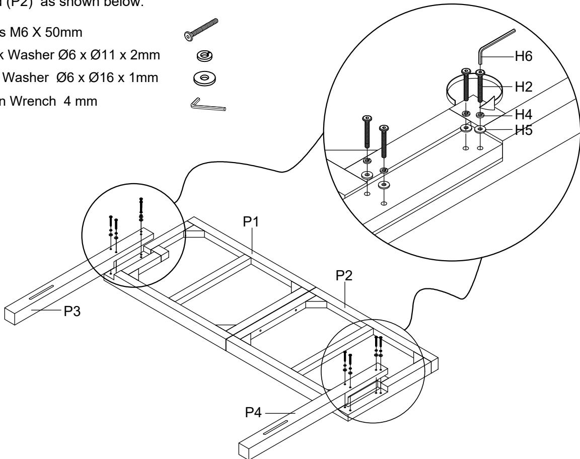
Step 3. Attach the connector plate (H7) to the right headboard (P1) and left headboard (P2) as shown below.
