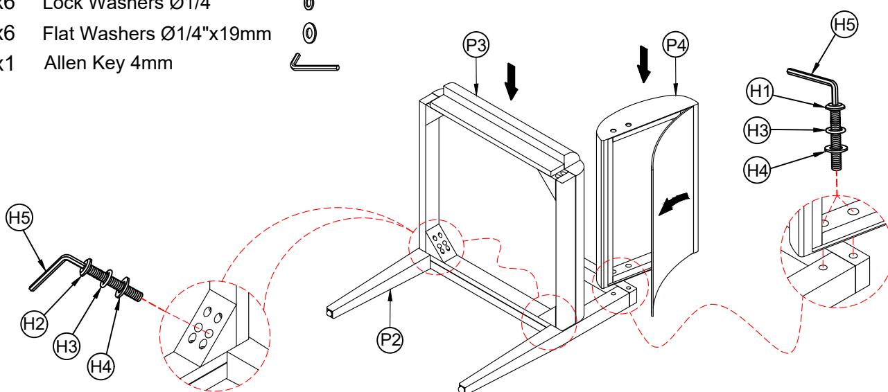
Step 2: Attach Right Leg Frame (P1) to Seat Cushion (P3) and Back Cushion (P4) as shown below. Tighten all bolts then close the Velcro of back cushion.
