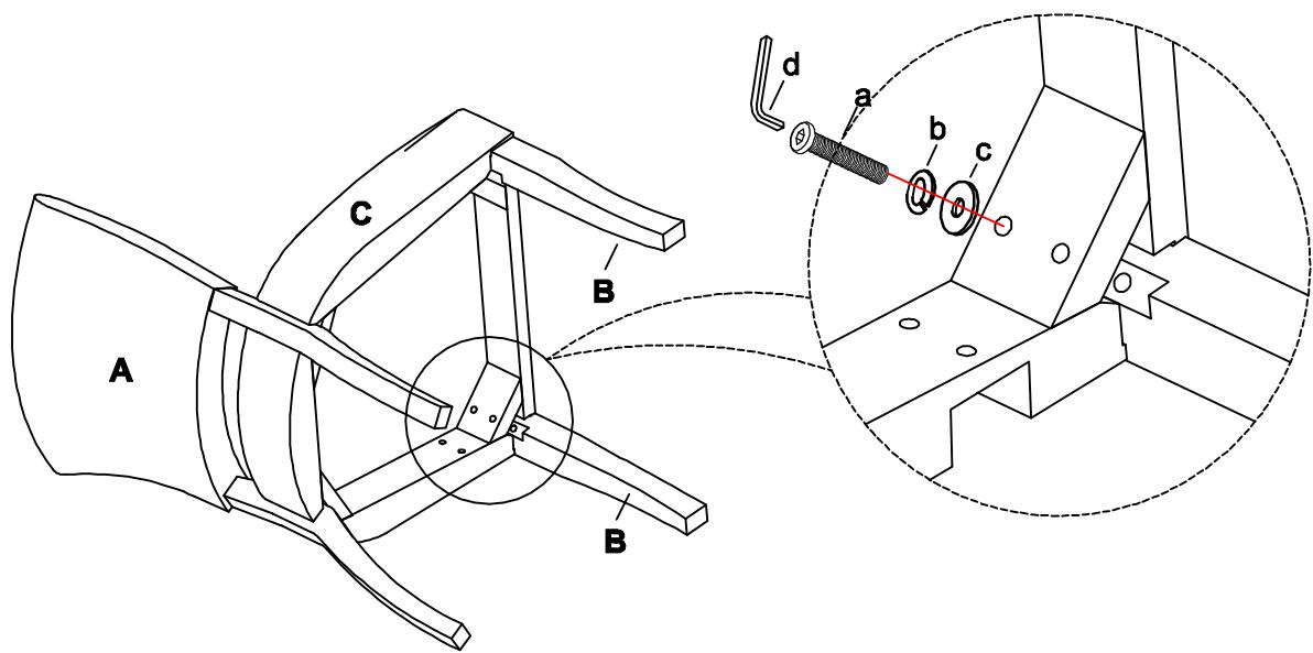
Step 3. Turn assembled the chair to an upright position. Securely tighten all bolts by Allen wrench (d). Assembly is complete. Failure to follow these instructions may cause the bolts to misalign during assembly.
