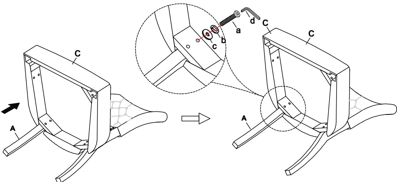
Step 2. Attach the front legs (B) to the seat cushion (C) using bolts (a), lock washers (b), flat washers (c). Loosely tighten the bolts with Allen wrench (d).
