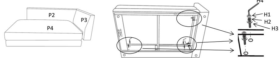
Step 4.Close the black fabric of the bottom.Screw in the legs (P1) using Plastic Washer (H5) for each. Screw tight to the right angle.
