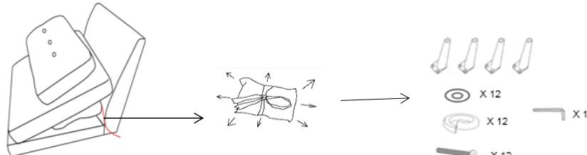
Step 2. Place the lounge(P2) onto a protective cloth. Using bolts (H1), lock washers (H2), flat washers (H3), connect legs(P1) to lounge (P2). Tighten bolts (H1) with Allen Wrench (H4).
