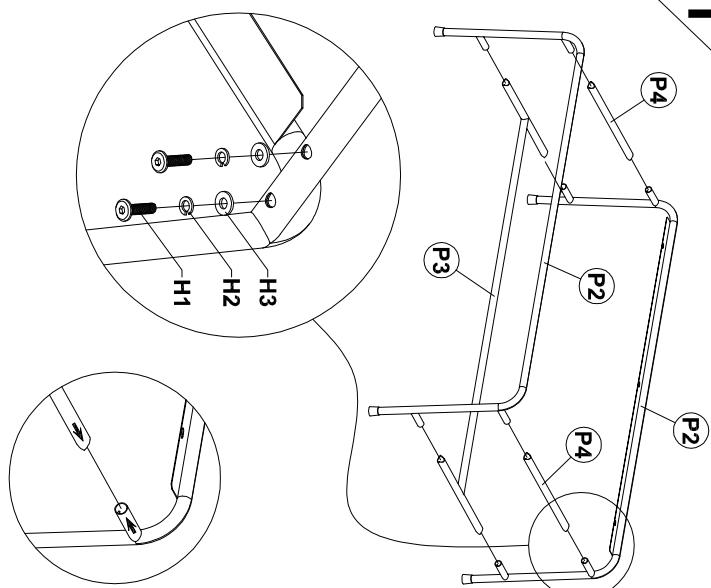
PLS, PLACE THE CONNECTOR HEAD RIGHT LOCATION WHEN ASSEMBLY. ARROW MARKED ON CONNECTOR WILL BE CONNECT WITH LOCATION HAVE ARROW MARKED ON FRAME. DONT TIGHTEN BOLTS UNTIL LAST STEP.
