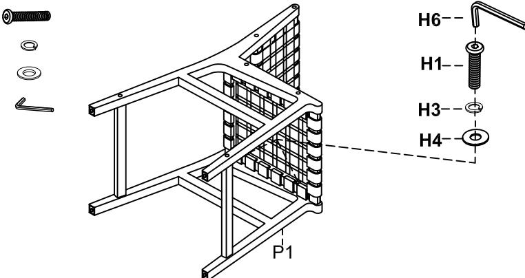
Step 5. Turn the assembled stool to an upright position, make sure the stool is level and securely tighten all bolts with Allen wrench (H6), then attach the wooden plugs (H7) to the left side frame (P1) and right side frame (P2) as shown. Assembly is complete.
