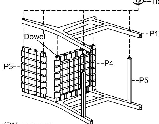
Step 4. Attach the seat panel (P4) to assembled left side frame (P1) as shown.
