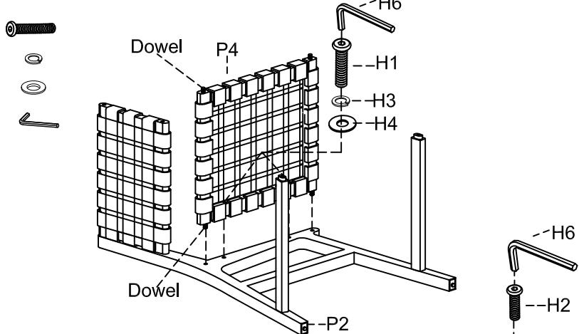
Step 3. Attach the left side frame (P1) to assembled back panel (P3) and seat panel(P4) and stretchers (P5) as shown.
