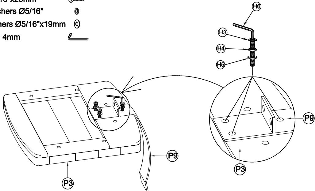
Step 3: Attach the assembled Leg frame to Seat Panel (P3) as shown below. Then tighten all bolts.
