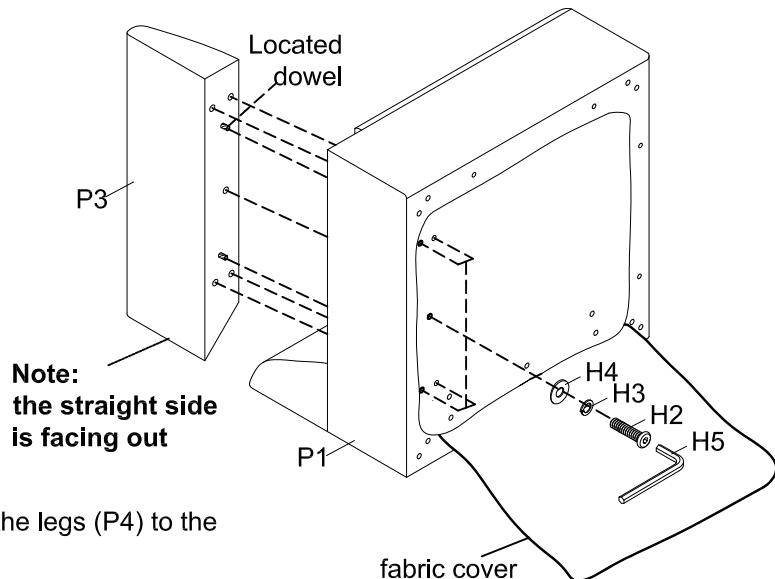
Step 3. Recover the fabric cover, then attach the legs (P4) to the bottom of seat (P1) as shown.
