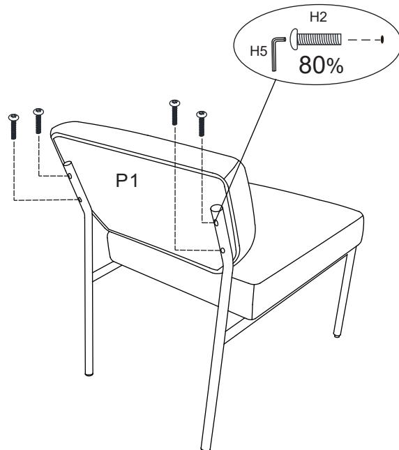
Step 3. Adjust levelers (as drawing) as necessary. Fully tighten the bolts as illustration below.
