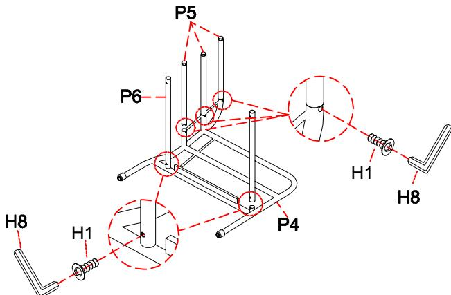
Step 2. Attach left arm (P3) to short rails (P5) and long rails (P6) as shown below. Securely tighten by small Allen wrench (H8).
