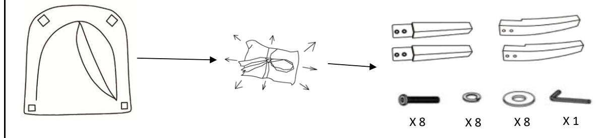
Step 2: Using flat washers (H3), lock washers (H2), bolts (H1), connect legs(P1&P2) to chair (P3). Tighten bolts (H1) with Allen Wrench (H4).
