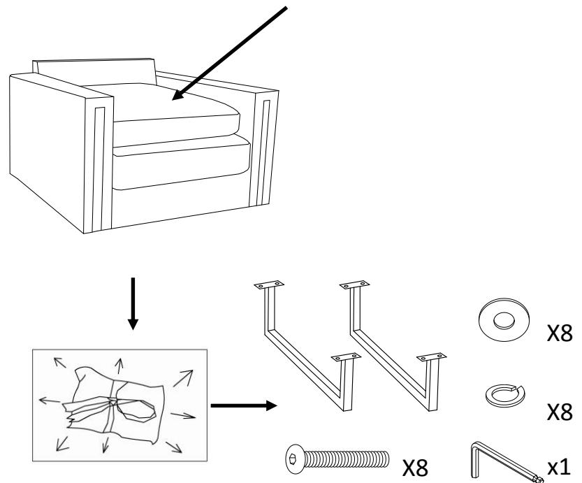
Step 2: Attach legs(P2) to the seat frame by using flat washer (H3),spring washer(H4), Long Bolt (H1)and use Allen wrench(H2)to tighten the bolt !
