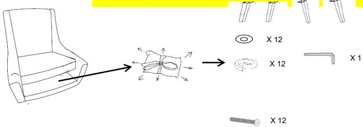
Step 2. Using bolts (H3), lock washers (H2), flat washers (H1), connect Front Legs (P2)(P3) and Back Legs (P4)(P5) to lounge (P1). Tighten bolts (H3) with Allen Wrench (H4).
