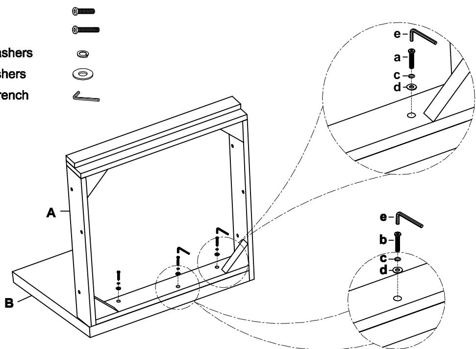
Step 2. Attach left arm (C) to the seat frame (A) and back frame (B) following the label "L" on the left arm (B), the side of seat frame (A) and back frame (B) accordingly as shown below. Securely tighten the bolts with Allen wrench (e) and (i).
