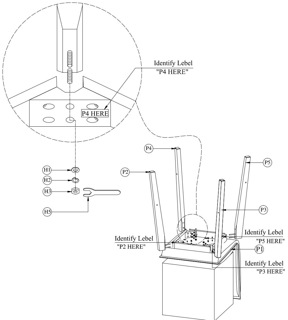
NOTE: DON'T TIGHTEN HEX NUT UNTIL ALL STRETCHERS WERE BEEN LOCATED INTO HOLES
