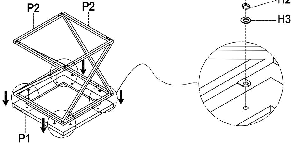
Step 4: Assemble the Adjustable Levelers (H5) as shown below:
