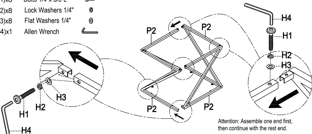
Step 3: Attach the assembled Metal Legs (P2) to the table top (P1) as shown below.
