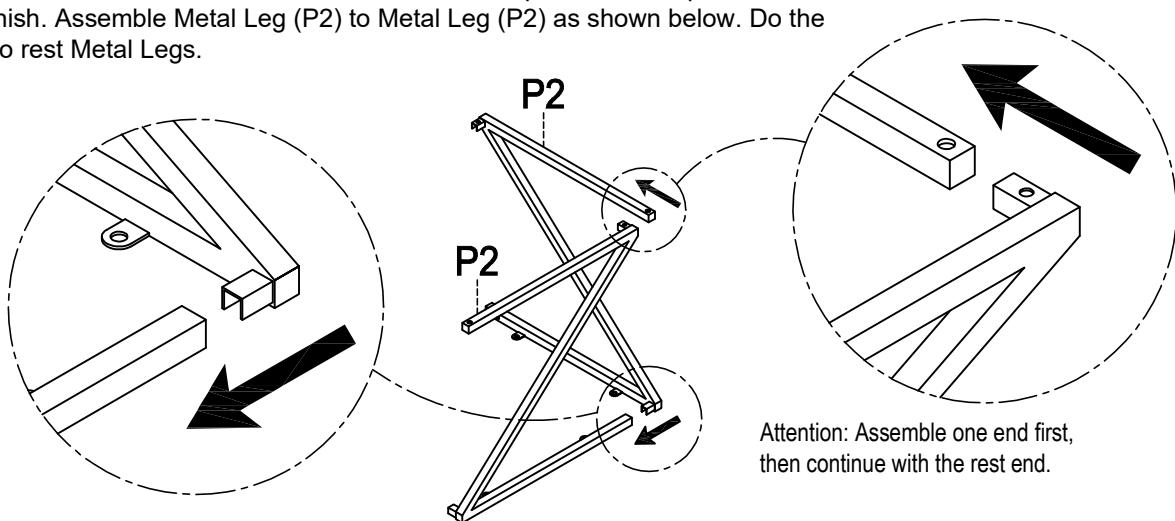
Step 2: Assemble Metal Leg Frames assembled in Step 1 together as shown below.
