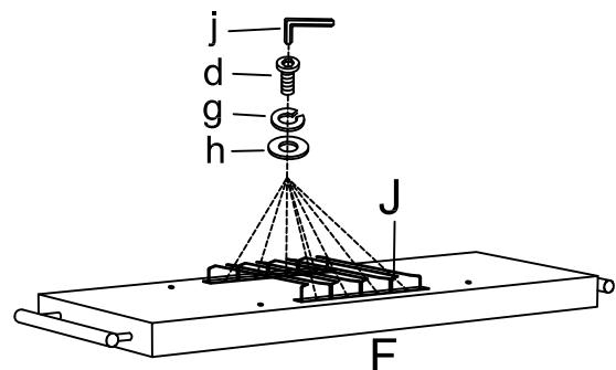
Step 8: Assemble the top tray (F) to the assembled base using medium short bolts (d), small flat washers (H), small lock washers (g) and small Allen wrench (j).
