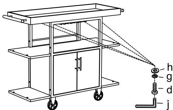
Step 9: Attach metal gallery (H) to the assembled base using bolt(c) and wrench(j).
