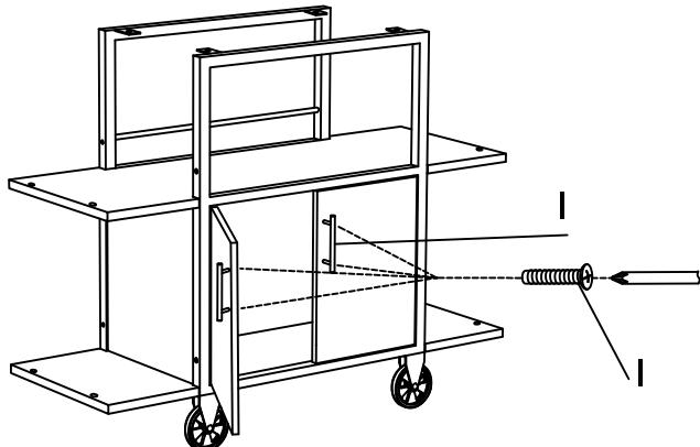
Step 6. Attach the big handle(G) to the top tray (F) by using medium long bolt (c) and small Allen wrench(j).
