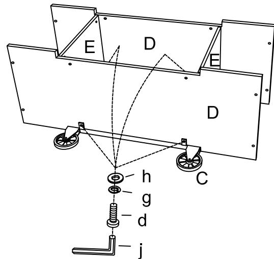
Step 4. Open the doors, then attach front frame (C) to the shelves (D) using medium short bolts (d), small flat washers (H), small lock washers (g) and small Allen wrench (j).
