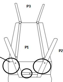
Step 4. Place the wood plug (H5) into the hole as illustration.
