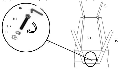
Step 3. Then using bolts (H1), lock washers (H2), flat washers (H3), connect wooden frame, **fully** tighten all bolts (H1) securely with allen wrench (H4) as illustration.
