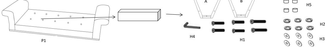
Step 2. Turn the bench (P1) upside down and lay on protective carpet. Attach the legs (P2&P3) to the bench, **loosely** tighten bolt (H1), lock washer (H2), flat washer (H3) with allen wrench (H4) as illustration below.
