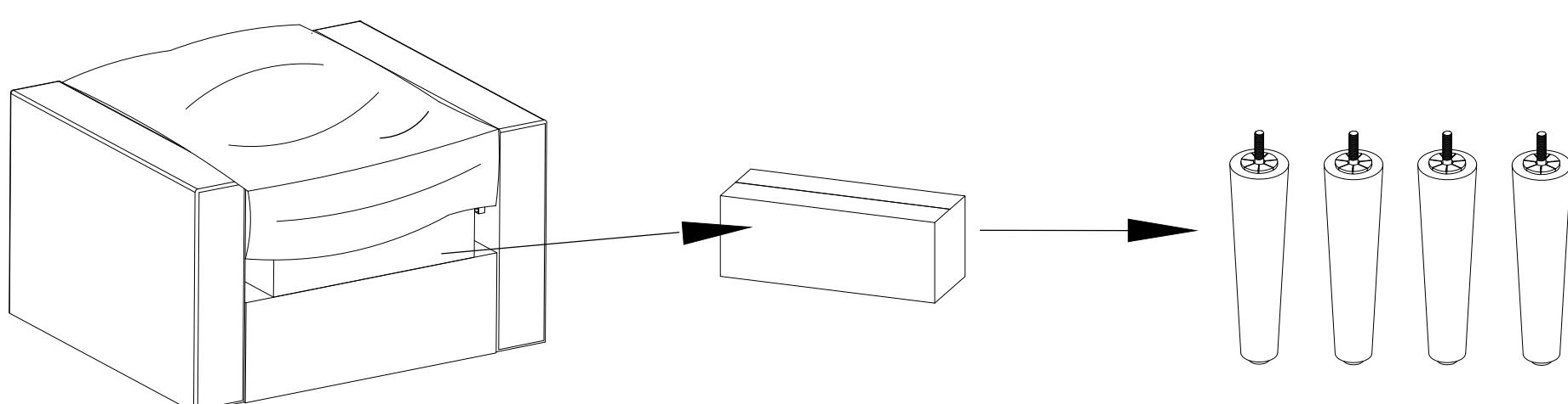
**Step 2:** Attach the legs (P1) into the holes on the bottom of chair seat (P5) through plastic washer (P2) as shown below:
